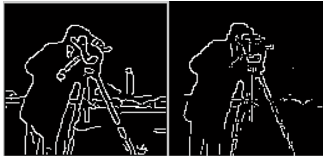
Fig. 3 Canny and Roberts Edge Detector outputs
