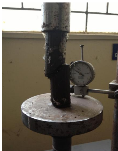
Fig.6 Specimen after failure
