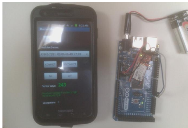
Fig.3: Android smart phone connected to Arduino Board via Bluetooth
