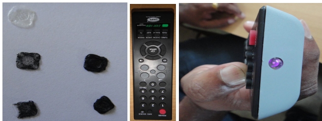
Figure 7. Testing of FC-CNP and FC-CNT in a Television (TV) remote control
