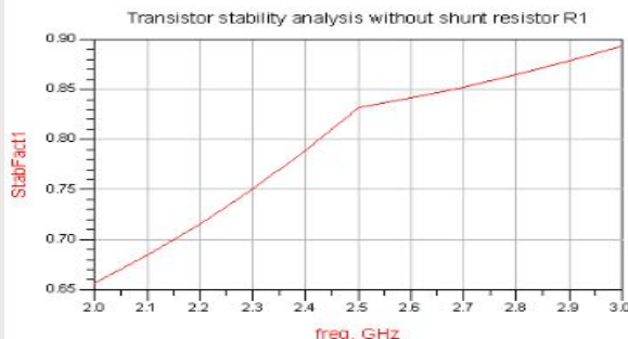
Fig 10. Simulation of Stability Analysis 1 ( K < 1 at 2.4GHz~2.5GHz)
