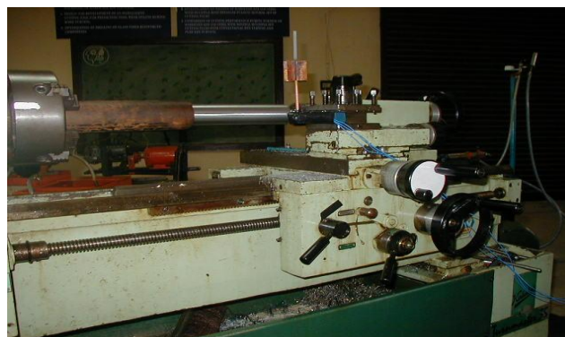
Fig 8. Experimental setup for with heat pipe
