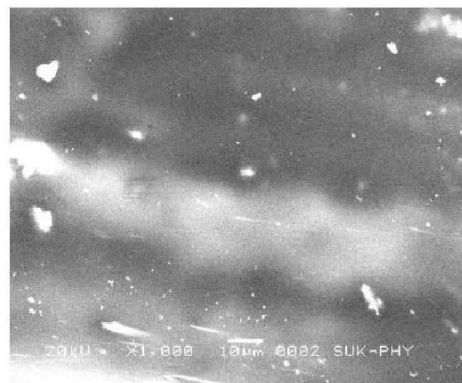
Fig.6. SEM images of worn surfaces with base oil with CuO nanoparticles
