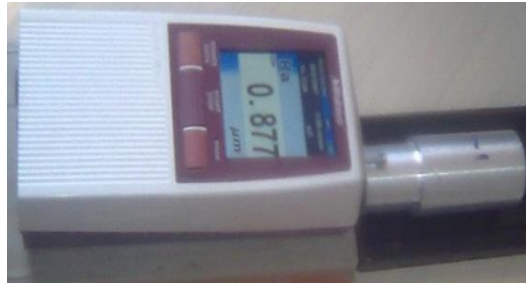
Fig: Measuring surface roughness of machined test specimen
