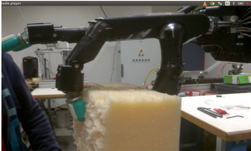
Fig 7 Precise Grasping by Shadow Hand using tactile feedback
