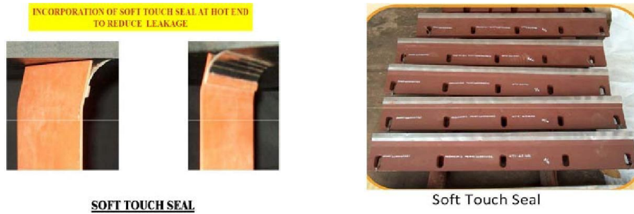
Figure 2: Incorporation of soft touch seal Figure 3: View of soft touch seal Diaphragm Plate Protection
