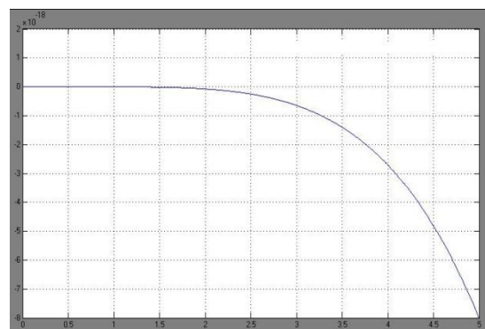
Fig.3.c (50-50-50 km.3 layer network output voltage with fixed supply voltage)
