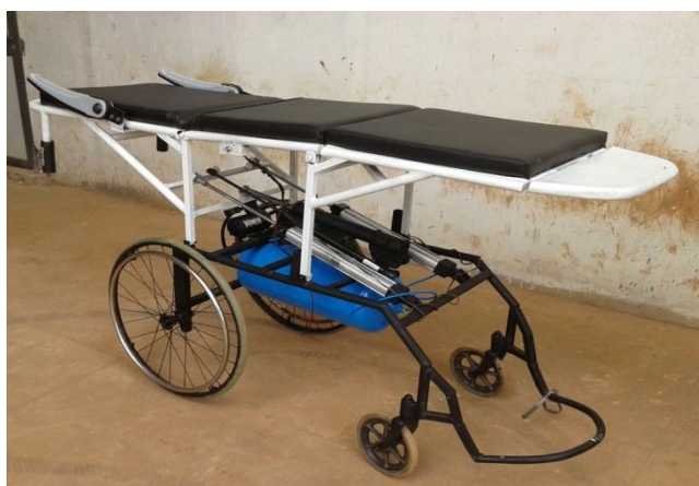
Fig.5.2: Image of the device in stretcher position
