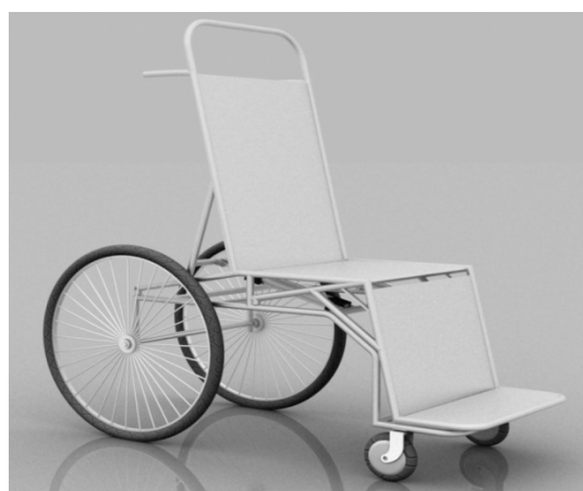
Fig.3.4: 3D view of the device in wheelchair position
