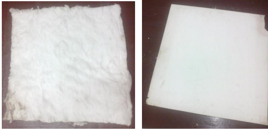
Fig.1.Ceramic Fiber and Silicon Fiber Sheet (Ceramic foam) dielectric materials respectively from left to right.
