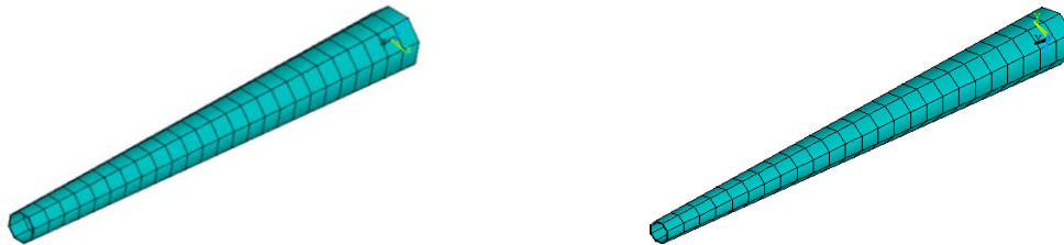
Fig 4: Cantilever beam (a) Before optimization (b) After optimization
