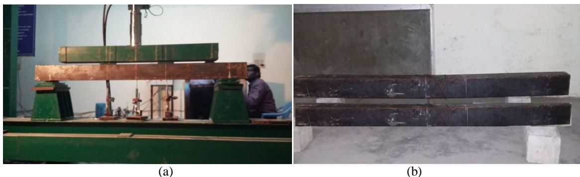
Figure 2 (a) shows the testing of a control beam and 2 (b) shows the control beams after failure
