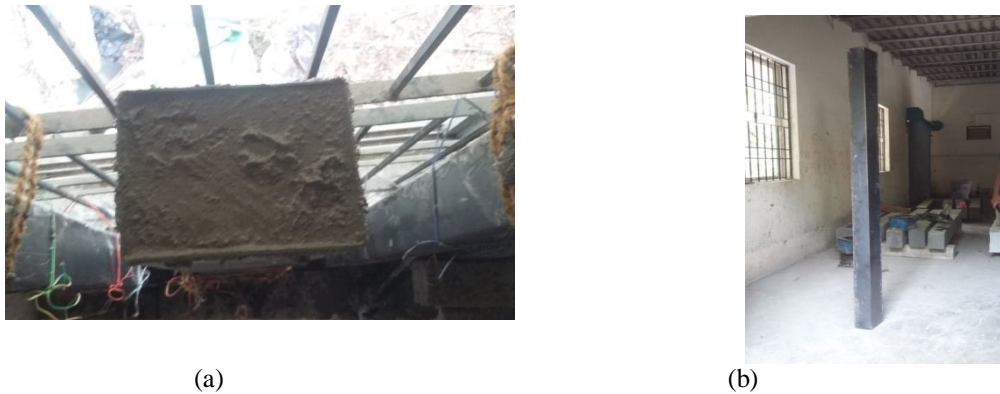
Figure 1 Casted CFST specimens (a) cross section of CFST specimens (b) shows the vertical section of CFST
