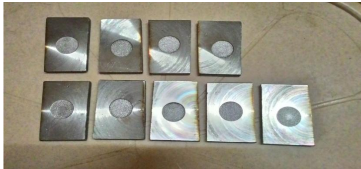
Fig. 3: AISI 316L stainless steel work piece after machining
