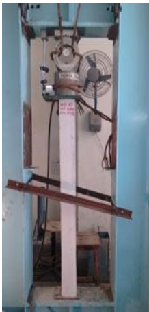
Fig 3: Test setup of a typical columns Fig 4: Cracked surfaces of failed column specimens
