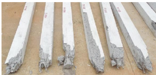
Fig 5: Crack and failure patterns of long columns
