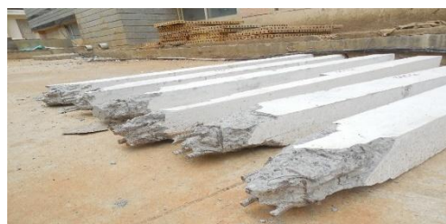
Fig 5: Crack and failure patterns of long columns
