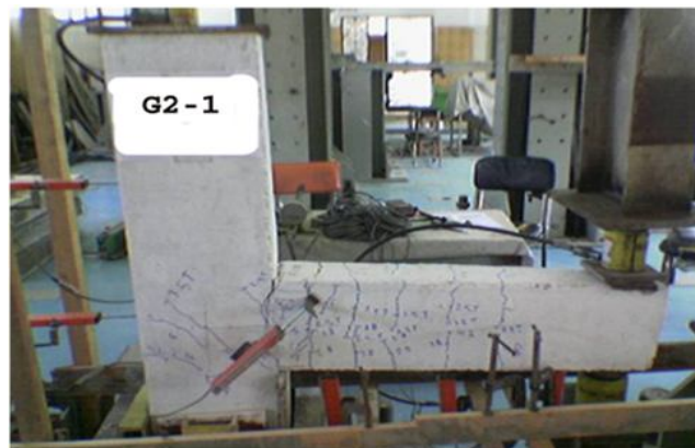
Fig.(6): Crack pattern and mode of failure for Specimen (1)
