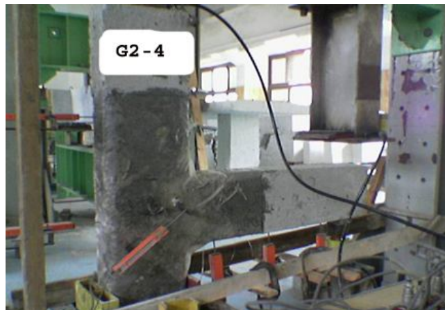
Fig.(9): Crack pattern and mode of failure for Specimen (4)
