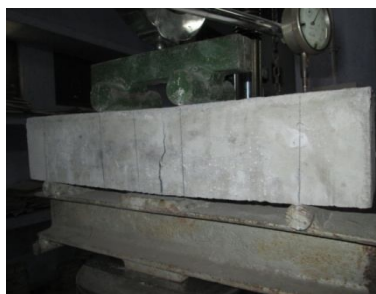
Fig : A typical arrangement for the measurement of flexural strength
