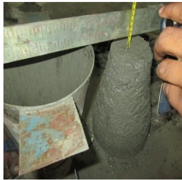
Fig: A typical arrangement for the measurement of slump
