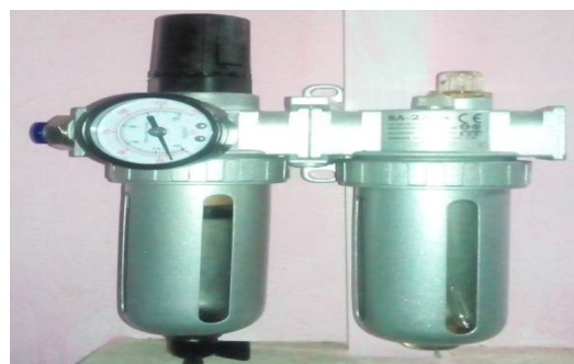
Photo No.2 FRL unit
