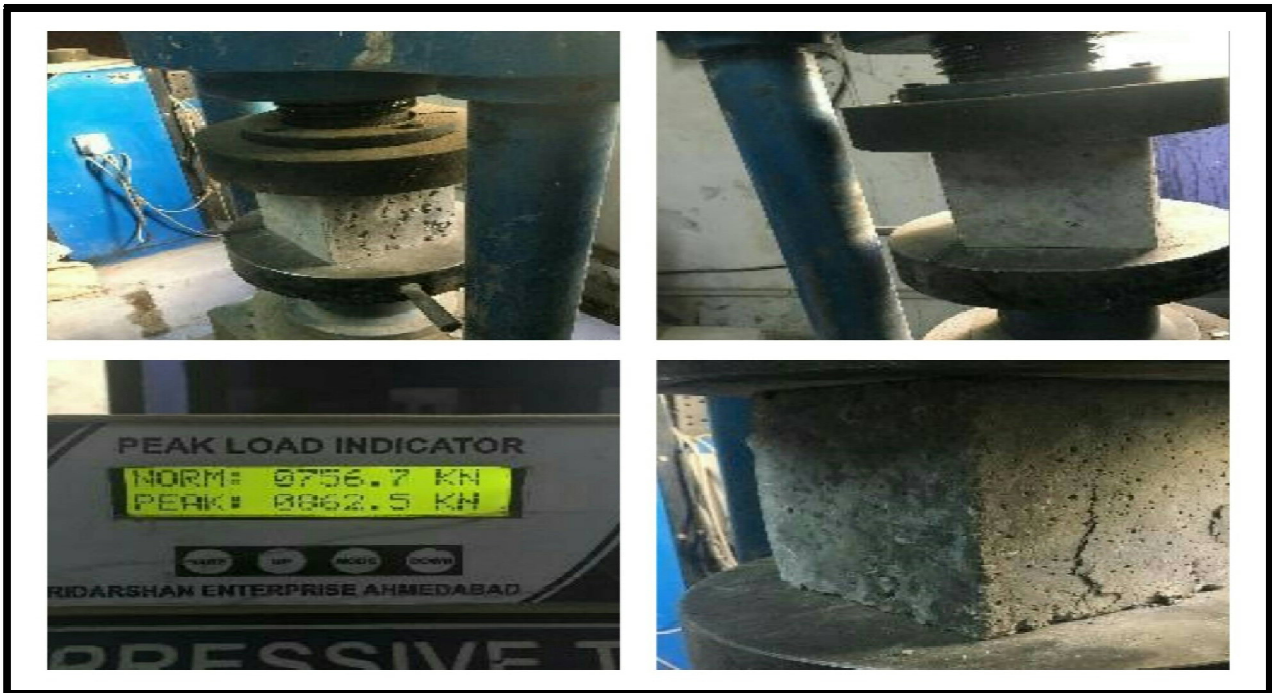
Figure:2 Compressive strength of cubes
