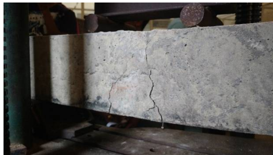
Fig 5: Flexural Strength Test
