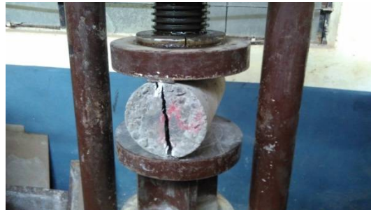
Fig 4: Split Tensile Test
