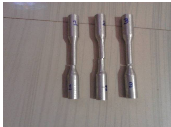
(b) Fractured tensile test specimens.
