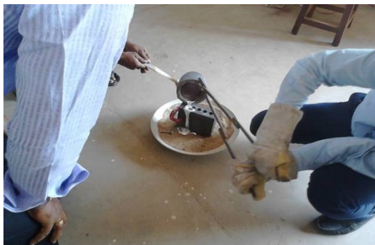
Fig (c) Pouring the molten metal into the S.G. Iron die
