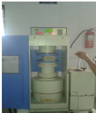
Figure 4: experimental set up for compressive strength test
