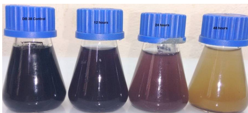
Fig. 1. Decolourization of the dye DB38 by Bacillus sp. KMSII-3 strain CSMB5
