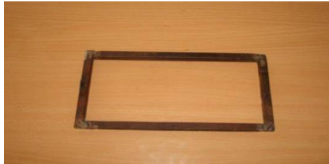
Fig. 3.1 Moulds for Making Composite Plates.
