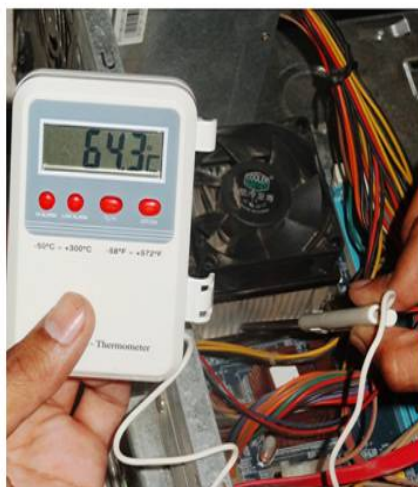
Fig. 4 Actual Temp reading of heat sink in CPU
