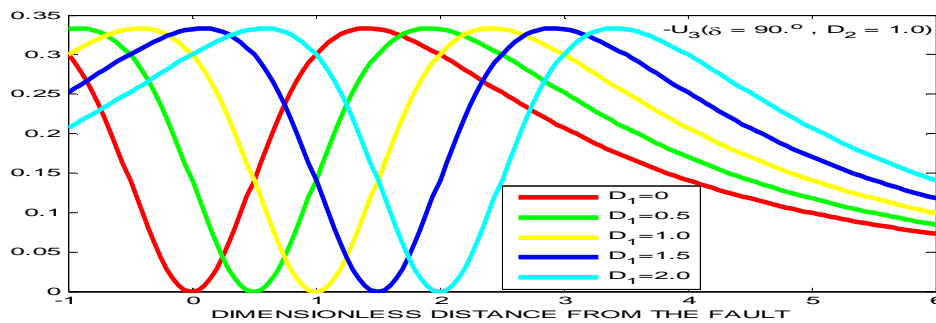
Figure 7: Variation of the dimensionless surface uplift -U_3 with distance from the fault for D_2 = 1.0 for (a) \delta = 0^\circ (b) \delta = 15^\circ (c) \delta = 60^\circ (d) \delta = 90^\circ .
