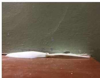
Fig 6. Fabricated 8045 standard propeller
