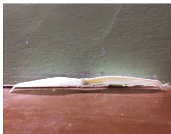
Fig 7. Fabricated 10 mm bent propeller
