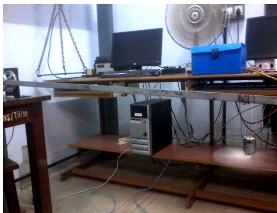
Fig 9. Experiment setup with contains torque trainer setup, motor and fabricated propeller
