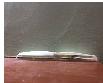
Fig 8. Fabricated 15 mm bent propeller
