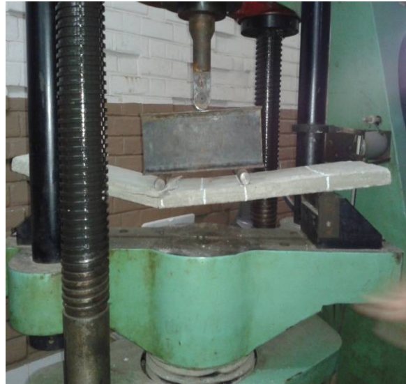
Fig-6: Panel Failure of 25 mm Thick
