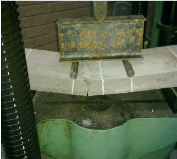
Fig-5: Panel Failure of 50 mm Thick
