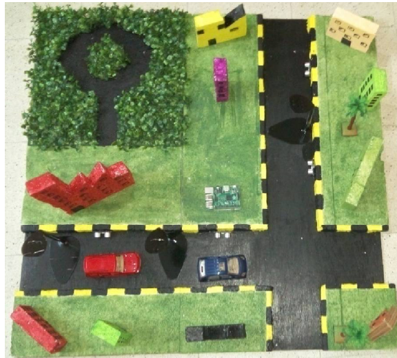
Fig 3. Top view of Model with Raspberry Pi 2 and ultrasonic sensors
