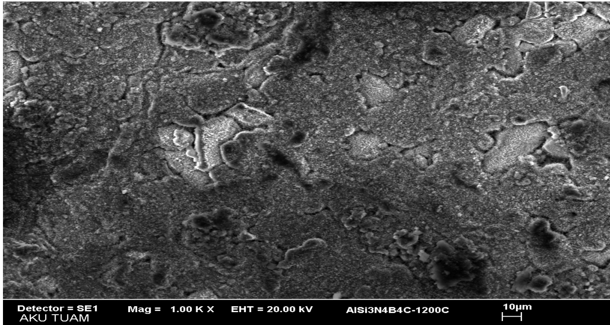
Fig. 3 SEM view of (%74Al-%9Ni-%9Al 2 O 3 -%4B 4 C-%4Si 3 N 4 ) composite 1200°C 1kX
