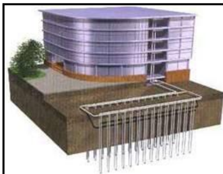
Fig-12 Stabilization by Heating Method
