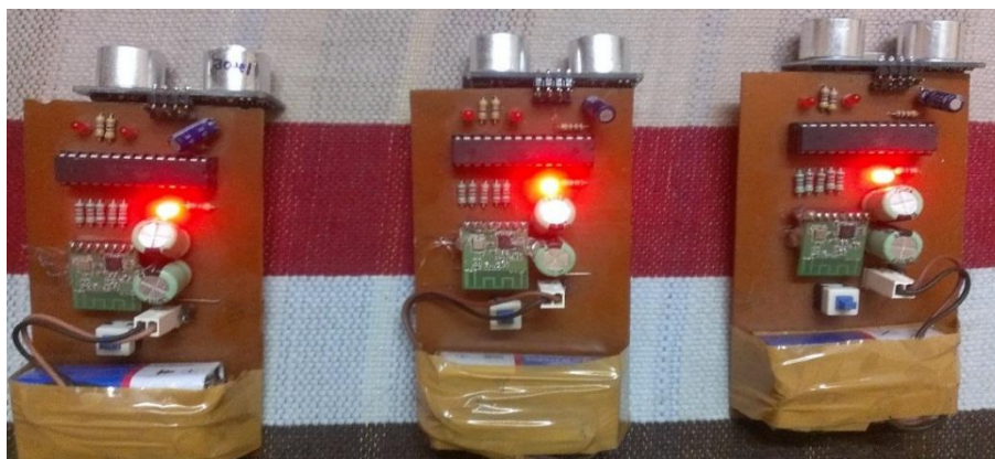
Fig.9 Multiple Ultrasonic Sensor
