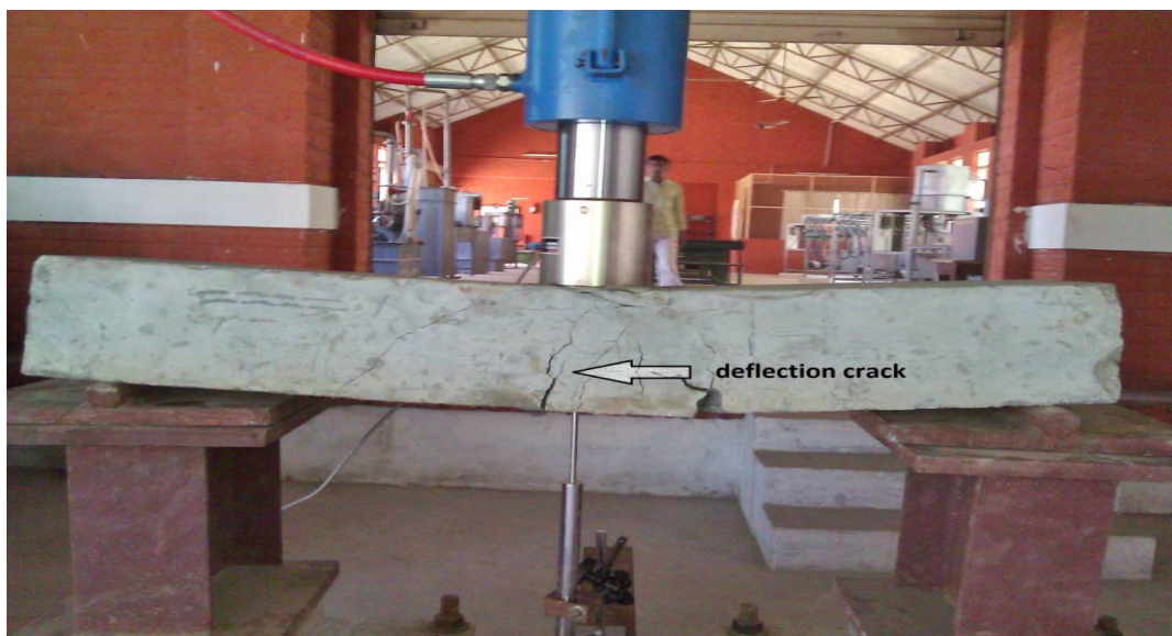
Figure 7: Shows arrangement and the loading of beam casted with TMT Rods with visible deflection crack at the middle and hairline cracks emerging from there onwards
