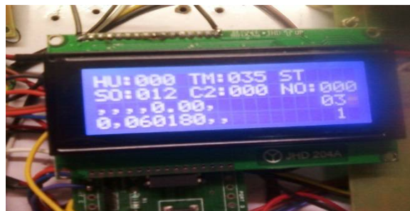
Figure 3. LCD frame showing pollutant levels
