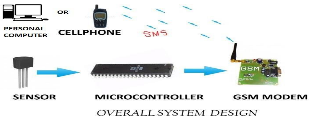
Figure 1. System hardware architecture
