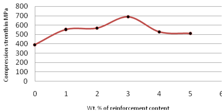
Fig. 8: variation of compression strength with increased content of Reinforcement in hybrid composites
