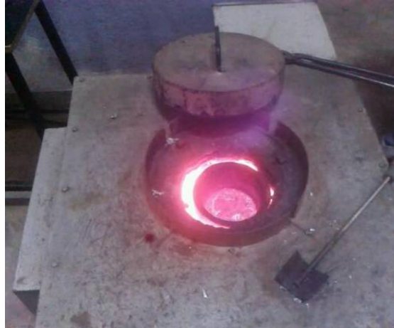
Fig. 2: Melting of Al2024 matrix material
