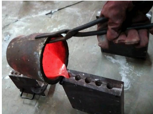
Fig. 4: Pouring of molten hybrid composites.
