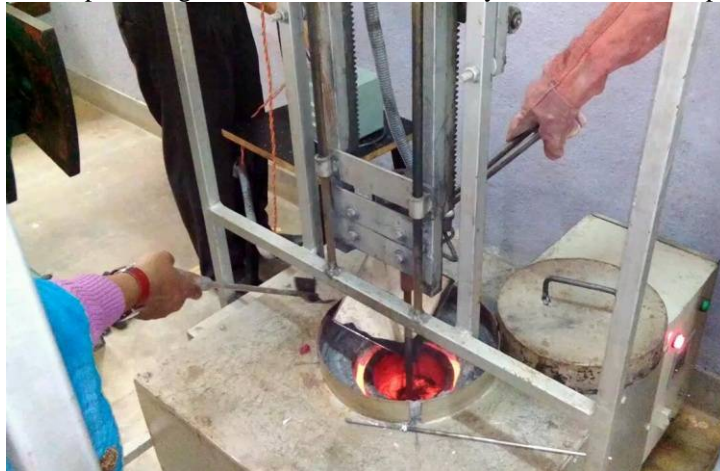
Fig. 3: Mixing and stirring of reinforcement material
