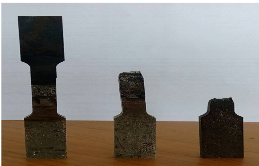
Fig 6 Tensile test specimen
