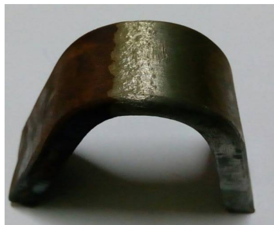
Fig 8 Root bend of weld joint
