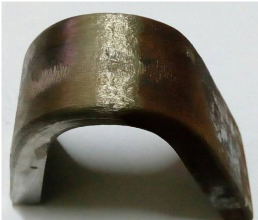
Fig 7 Face bent of weld joint
