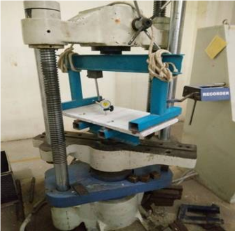
Tabulation for Flexural test on test specimen with cement-copper slag
