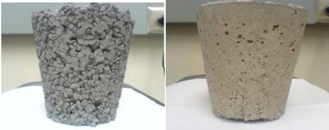
Figure 3.6. a) Porous castable prepared from virgin castable mix b) dense castable prepared from normalized castable mix of type I refractory.
