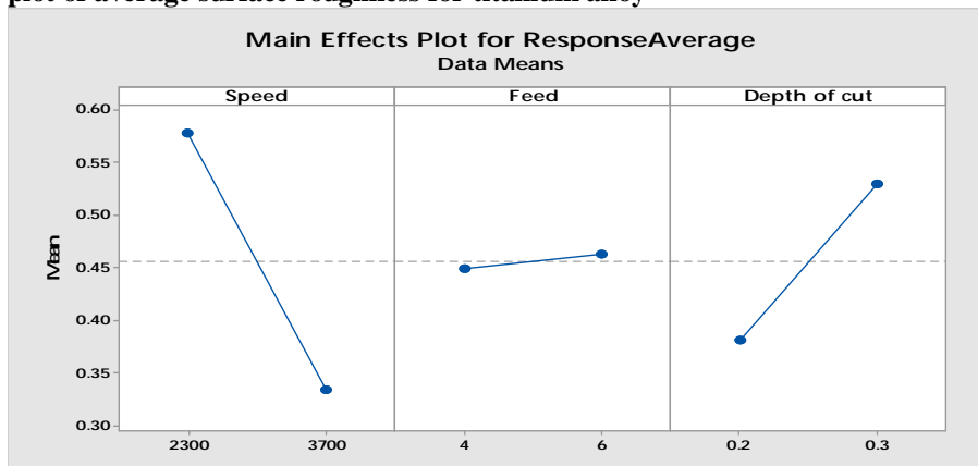
Fig 4. Main effects plot of average surface roughness for titanium alloy
