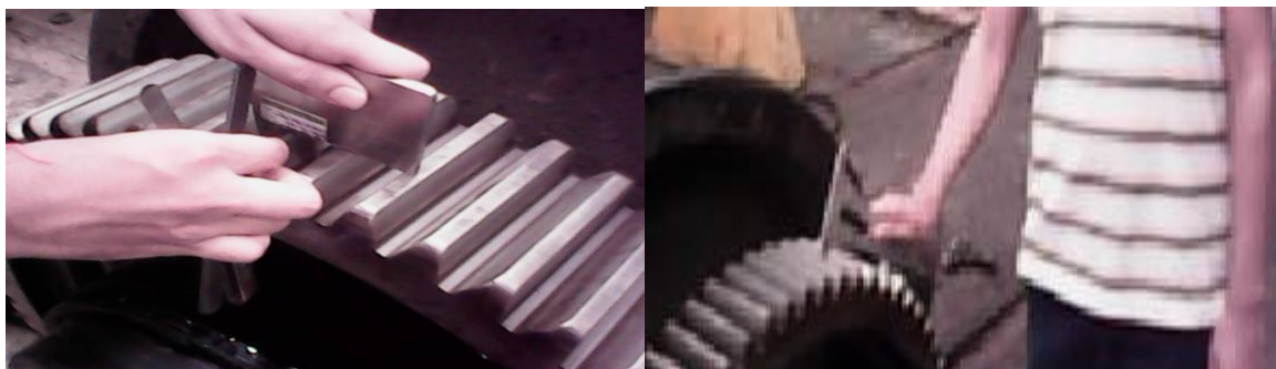
Fig. c. Measurement of P-Value, K-Value and Backlash of Axle Gear Box
