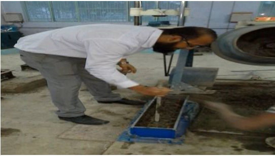
Hand compaction of beams
