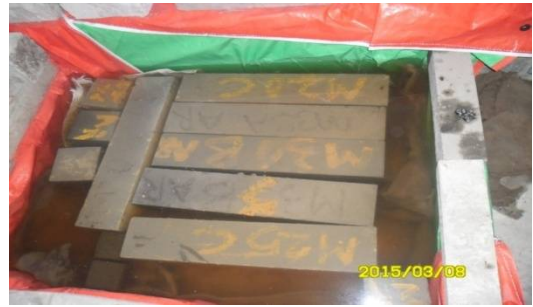
Water tank for curing of specimens
