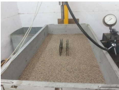
Figure 3: Placing of Piles in appropriate positions
