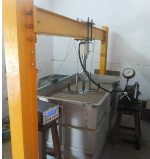
Figure 5: Experimental Setup of Piled Raft Foundation
