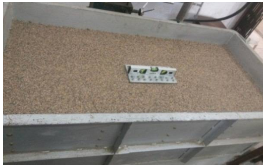
Figure 2: Preparation of Sand Bed
