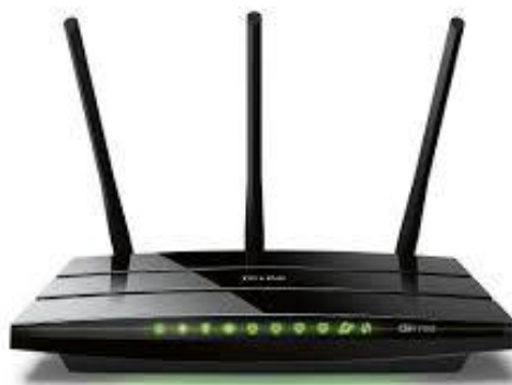
Figure 1: Router Device: A networking Device that forward data packets.
