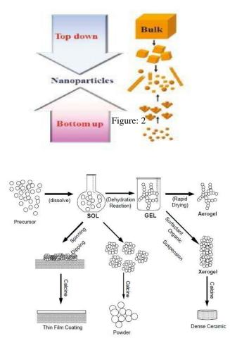
Figure 3. Sol-gel processes for synthesis of nanomaterials.
