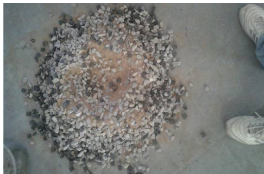
Fig1: Mixing of scrap tyre rubber in concrete
