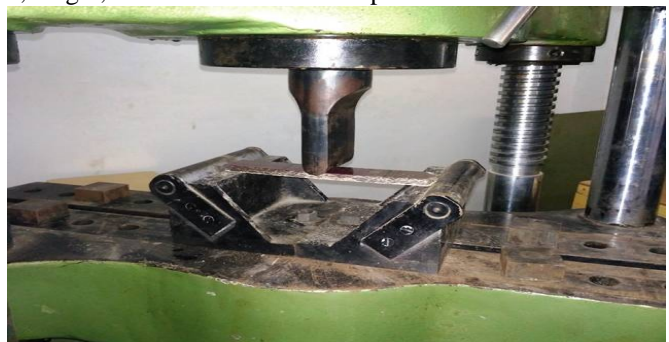
Fig.17. Flexural test on sample K15J85
