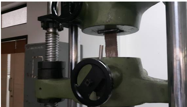
Fig.3. Tensile test on Jute specimen strips
