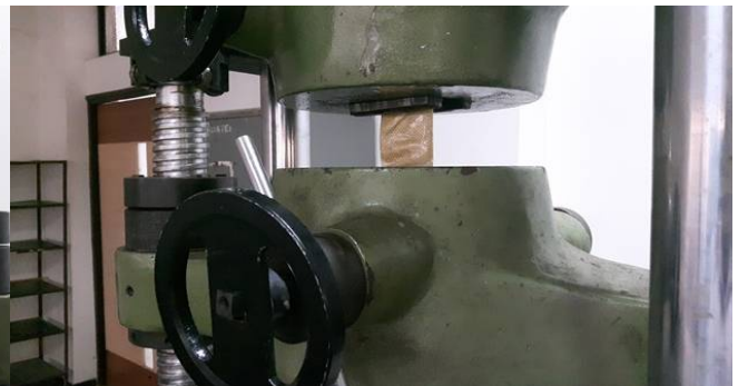
Fig.4. Tensile test on Kevlar specimen strips
