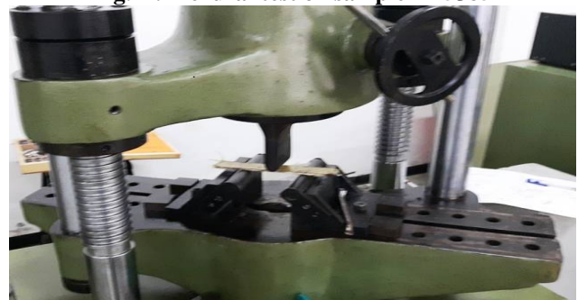
Fig.19. Flexural test on sample K75J25
