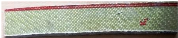
Fig.8. Tensile test specimen (K15J85)
