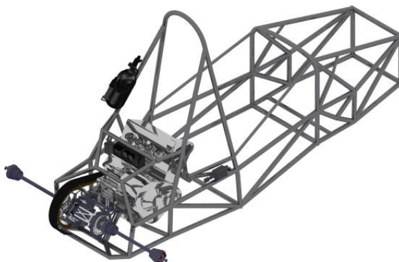
Fig. 2(c) Transmission assembly mounted onto the chassis
