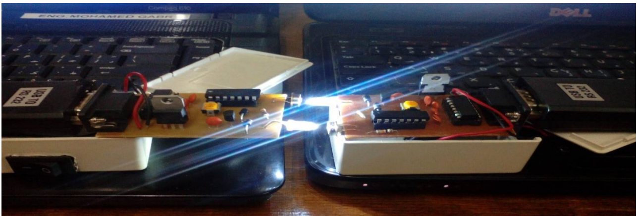
Fig. 5 (b) VLC System (the same system above ) after connecting power to both circuits
